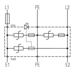
IEC 61643-11 AS/NZS 1768 UL 1449 IEEE 62.41.2 SPD connected to low-voltage power systems - Type 2 + 3
