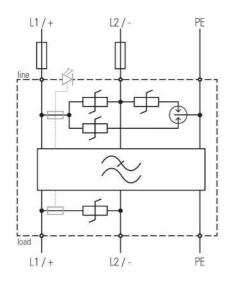
IEC 61643-11:2011 AS/NZS 1768:2007 UL 1449 3rd edition IEEE 62.41.2:2002 SPD connected to low-voltage power systems - Type 2+3 A.C. power system SPD - Cat C, B, A Low voltage SPD - Type 2, 3 Low voltage SPD - Cat B
